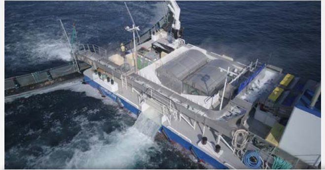
New thermal and mechanical treatment options involve vessels like the Hydrolicer, where fish are put through pressurized freshwater or warm water baths. Despite the hype, these novel methods have been unable to control sea lice outbreaks to-date. Photo: Hydrolicer
