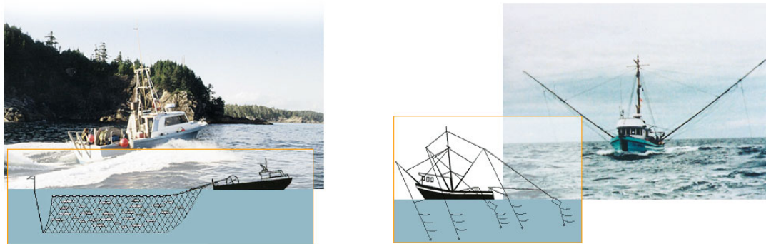
Figure 4.1. Driftnet and troll gear types ( www.goldseal.ca/ ).
